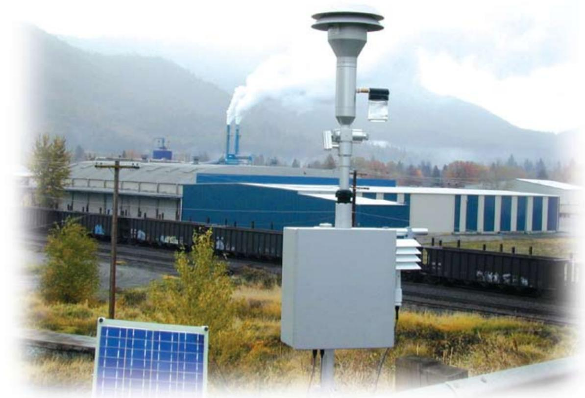
The Met One E-BAM is a portable, real-time beta gauge which is comparable to U.S. EPA methods for PM<sub>2.5</sub> and PM<sub>10</sub> particulate measurements.
